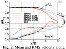
Fig. 2. Mean and RMS velocity along the jet centerline, effect of different SEM parameters
