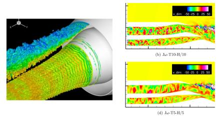
Fig. 3. Dual stream jet, simulations with different upstream turbulence parameters. Left: Q-criterion isosurface, right: contours of radial velocity.
