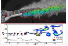
Fig. 1. Illustration of a simulation with upstream turbulence, focus on the mixing layer development
