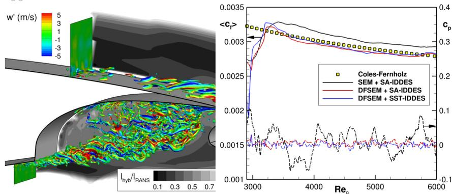
**Fig. 1** Left: Injection of synthetic turbulence in two planes of a multi-element airfoil flow. Right: Mean skin friction and instantaneous pressure on a flat plate.
