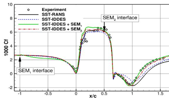
**Fig. 2** Mean skin friction along a 2D wall-mounted hump.
