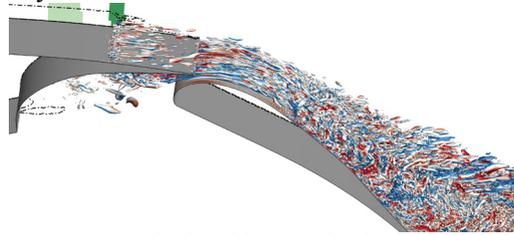
**Fig. 2** Turbulent structures depicted by Q-criterion, forcing region in green.
