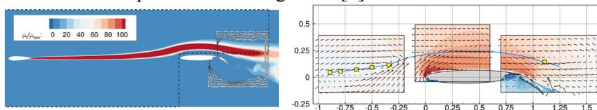
**Fig. 1** Simulation setup: viscosity ratio indicates RANS and LES regions (left). Three positions of the vortex passing the HL airfoil (right).
