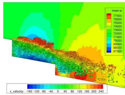
Fig. 4: Q isocontours using SST-IDDES
