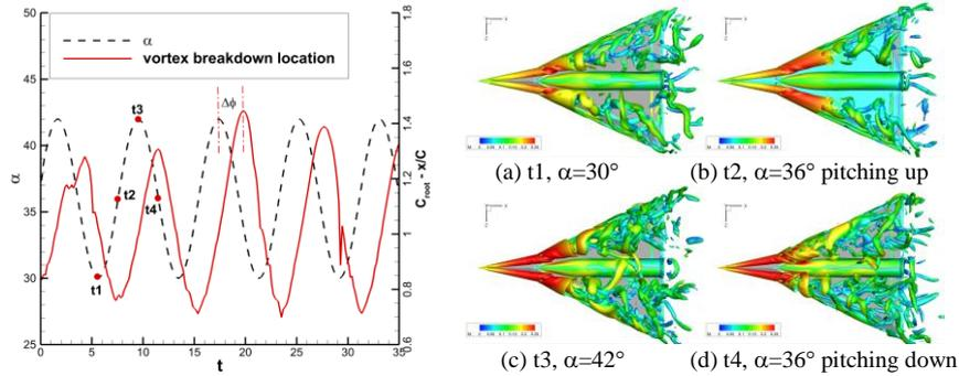
**Fig. 2** The lag between burst point and incidence( $k=0.4, \alpha_m=6^\circ$ )
