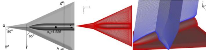
Fig. 1 Model and Mesh of  $80^\circ/65^\circ$  double-delta wing
