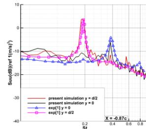
**Fig. 2** Comparison of streamwise velocity spectra between present simulation and the experiment.
