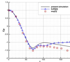
**Fig. 1** Comparison of pressure coefficients on rod-surface between present simulation and the existing literatures
