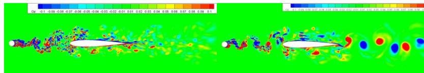
**Fig. 3** Comparison of the spanwise vortices between the stationary configuration and oscillating one (left: stationary; right: oscillating)
