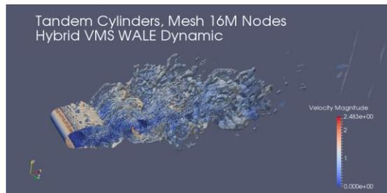
**Fig. 2** Tandem cylinders at  $Re=166K$ : instantaneous iso-surfaces of  $Q$ -criterion field colored by velocity magnitude (Hybrid VMS Dynamic).
