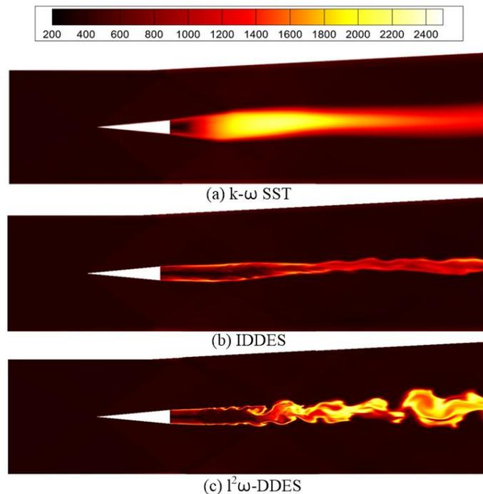
Fig. 1 Static temperature contours for each turbulence models
