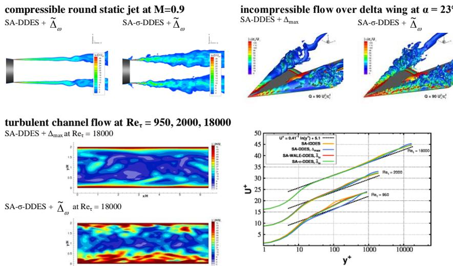
**Fig. 1:** Comparison of performance of improved  $\sigma$ -DDES relative to standard DDES for various complex test cases.
