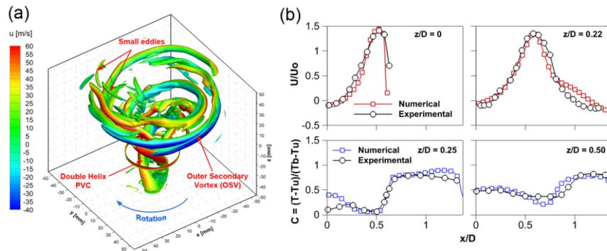
**Fig. 2** 3D flow structure (a) and validation with measurements (b)
