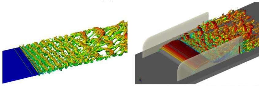
**Fig. 1** Visualization of resolved turbulent structures for a mixing layer (left) and for the separated flow behind the NASA Hump (right)
