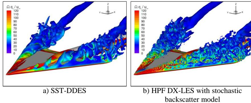
**Fig. 1** NASA delta wing at high angle of attack: iso-contours of Q-criterion coloured with vorticity magnitude
