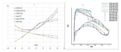
Fig. 1 k- $\omega$  SST RANS for AVM-DZ vs experimental results. Aerodynamic coefficients (a) and Cp plots for AoA = 2.45 deg.(b).
