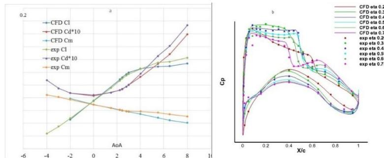
Fig. 1  $k-\omega$  SST RANS for AVM-DZ vs experimental results. Aerodynamic coefficients (a) and  $C_p$  plots for  $AoA = 2.45$  deg.(b).
