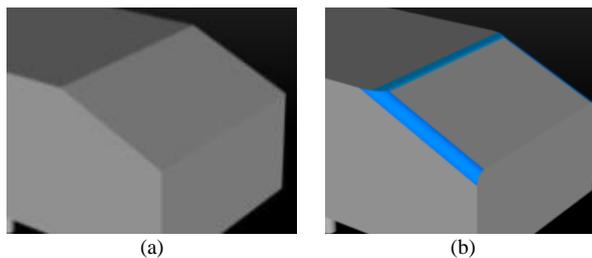
**Fig. 1** (a) 25° Ahmed body with sharp edges and (b) 25° Ahmed body with rounded edges, in blue
