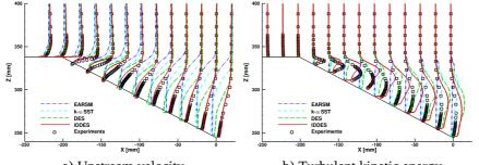
a) Upstream velocity b) Turbulent kinetic energy **Fig. 1** Comparison of U component and TKE in th symmetry plane
