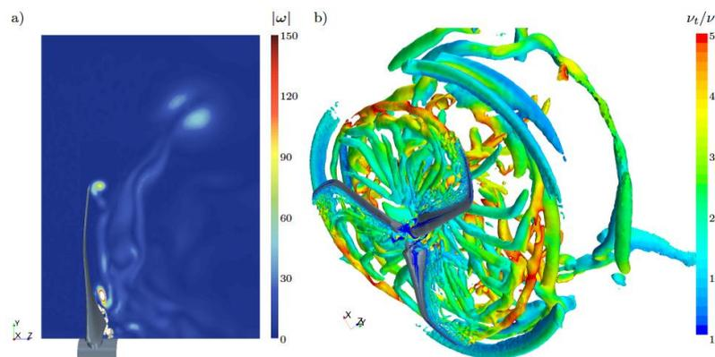
**Fig. 2** Contour plot of instantaneous vorticity magnitude (a) and iso-surfaces of Q-criterion (b), coloured by the ratio of turbulent eddy- and kinematic viscosity.
