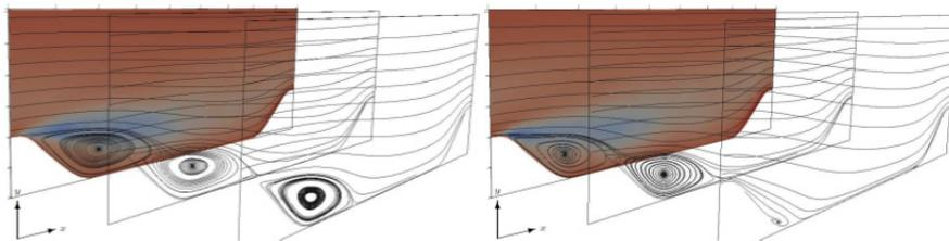
**Fig. 2** Wall-resolved periodic hill flow for different resolution ( $N_x \times N_z = 148 \times 92$ ,  $128 \times 80$ ,  $98 \times 64$  from left to right in each sub figure using EASSM (left) and DSM (right). Mean streamlines and colours by resolved  $\overline{u'v'}$ . Figure is taken from [5].
