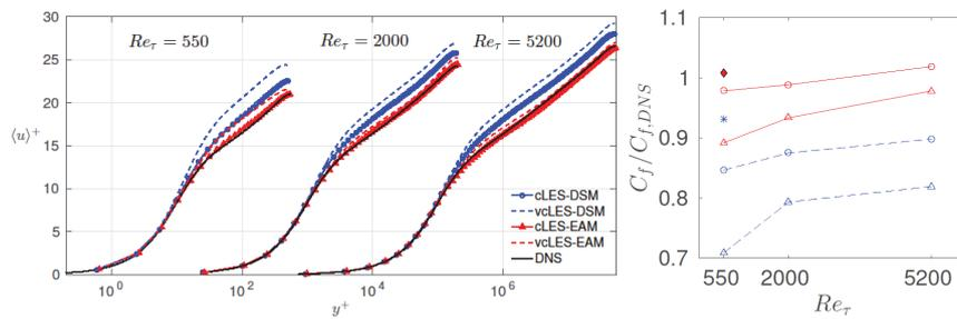
**Fig. 1** Wall-resolved LES of plane channel flow for different resolutions ( $\Delta_x \times \Delta_z \approx 150 \times 60$ (c,  $\circ$ ),  $250 \times 100$ (vc,  $\Delta$ )) at different  $Re$  using EASSM & DSM.
