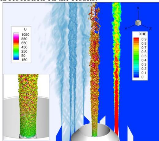
**Fig. 1** Preliminary results with translated numerical Schlieren slice (left), isosurface of Q-criterion coloured by x-velocity (center), translated Helium molar fraction slice (right)
