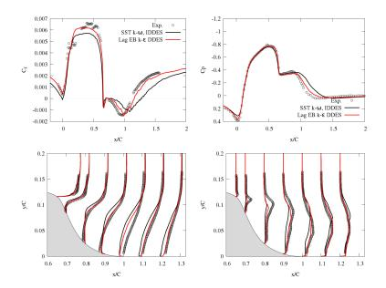
Fig. 1 Comparison of (from left to right, and top to bottom), the skin-friction coefficient, the pressure coefficient, the streamwise velocity and  $\overline{uu}_{tot}/U_{\infty}^2$ , between the SST  $k - \omega$  IDDES and the Lag EB  $k - \varepsilon$  DDES model. The velocity fluctuations include both modelled and resolved contributions.
