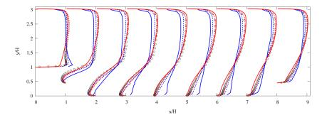
Fig. 2 Periodic hill flow: (top) meshes used for the RANS solution (red) and the LES (blue). Bottom plot: averaged RANS (solide blue line) and LES field without drifts terms, and with drift terms (dashed lines).
