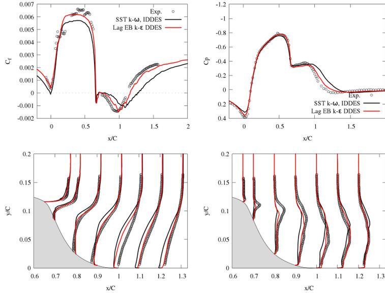
**Fig. 1** Comparison of (from left to right, and top to bottom), the skin-friction coefficient, the pressure coefficient, the streamwise velocity and  $\overline{u'u'}/U_\infty^2$ , between the SST  $k-\omega$  IDDES and the Lag EB  $k-\varepsilon$  DDES model. The velocity fluctuations include both modelled and resolved contributions.
