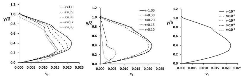
**Figure 1:** Eddy-viscosity profiles for DES(left) and DDES(middle) and SBES (right)under grid-refinement. (Note that range for SBES goes from  $r=1-10^{-4}$ ).
