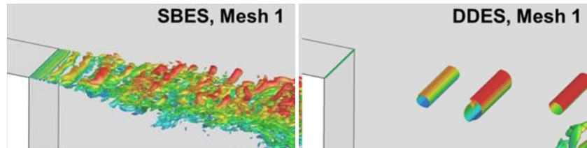
Figure 3: Iso-surfaces of the  $Q$ -criterion coloured with the velocity magnitude. Left SBES, right DDES
