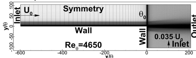
Figure 2: The domain and grid for the single stream mixing layer flow
